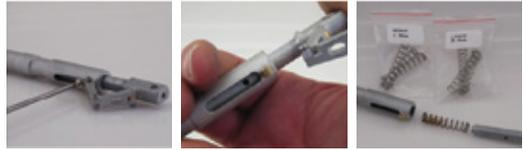
7. Test the units for correct and clear operation, making sure the retract struts or wheels does not come into contact with the plane structure during the retraction cycle and there are no obstructions in the wheel wells.
