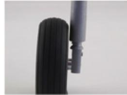
4. Insert the retract unit into the wing and fasten the mounting screws ensuring the wheel does not make contact with any of the wheel well sides.
