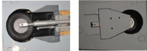
Ensure to use main gear struts, which are easily identified because they are solid on the top and has no hole for the steering pin like the nosewheel does.
