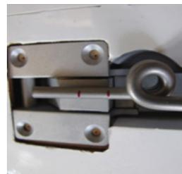
3. Grind two flat spots on both sides of the strut to enable the grub screws in the trunnion to lock securely. Insert and lock the strut properly into the Trunnion first before bolting the retract unit into the wing.
