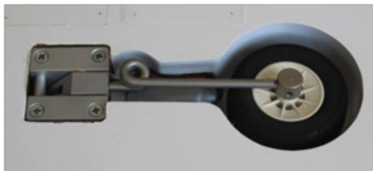
7. Test the units for correct and clear operation, making sure the retract struts or wheels does not come into contact with the plane structure during the retraction cycle and there are no obstructions in the wheel wells. Leave the wheels out and assemble your plane to enable you to determine the appropriate nosewheel strut length.
