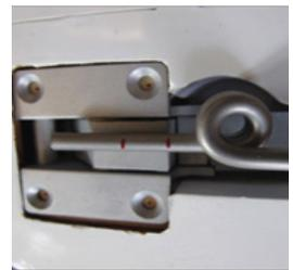
3. Grind two flat spots on both sides of the strut to enable the grub screws in the trunnion to lock securely. Insert and lock the strut properly into the Trunnion first before bolting the retract unit into the wing.
