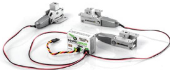
A. Plug the connector from each gear into the slots marked Gear on the ACE controller. Note correct polarity of the plugs, incorrect connections will not damage the ACE unit but the retract units will not work at all until correctly installed. Install the ACE controller in an area where it will not be exposed to any fuel, oil or moisture.
