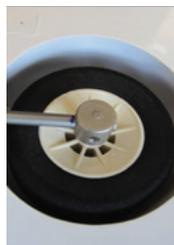
4. Slide the wheel onto the axle and make sure it has a secure fit. If the wheel hole is too small, drill it out to the correct size. If the wheel hole is too big, you can get a piece of brass tubing that slide over the axle and drill the hole in the wheel(if needed) to secure a good fit with the tubing.
