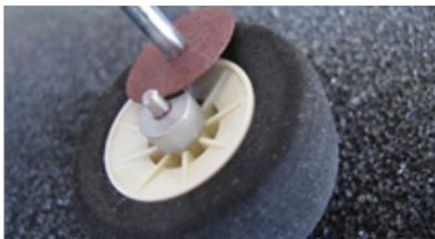
5. Slide the wheel axle onto the strut and determine the correct center point at the center of the wheel well and mark that position. Remove the wheel axle and determine the center of the 2 marks for the axle. Grind two flat spots on the center mark of the strut where the axle needs to be secured to the strut. Cut the remainder of the strut that would not be needed off and install and fasten the wheel axle properly.
